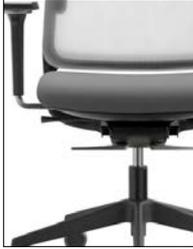
**SYNCHRO ATOM:** rotation of the backrest relative to the seat, with the rotation center located above the seat surface, ensuring an optimal movement during the reclination. Height adjustment by a handle. The mechanism tension adapts automatically to the weight of the user (for people between 45 and 110 kg). The backrest may be fixed by using a handle. As option, there are five different positions to adjust the seat depth or Trasla.
